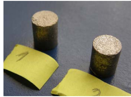
Fig. 9. Composites with 70% 316L and 30% Hap.
